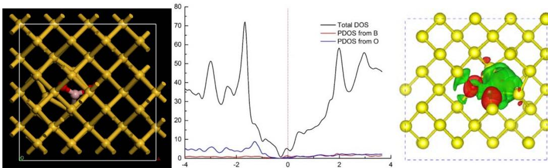
Structure, density of states and electron redistribution after BO<sub>2</sub> is introduced (both B and O are interstitial). The electronic distribution is defined as  $\rho_{\text{tot}} - \rho_{\text{BO}_2} - \rho_{\text{bulk-si}}$ , red: electron gain (mainly on O atoms); green: electron loss.
